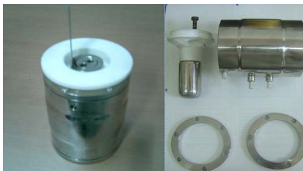
Fig. 2 Photographs of the coaxial cylinder electrode treatment chamber
